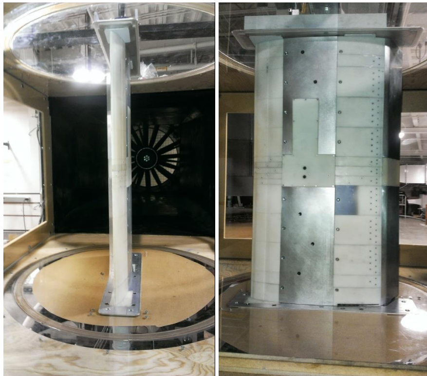
Figure 13. Airfoil assembly in test section with attached turning system
