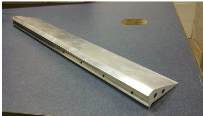
Figure 20. Airfoil aluminum: (a) Top and bottom core, and (b) right and left trailing edge
