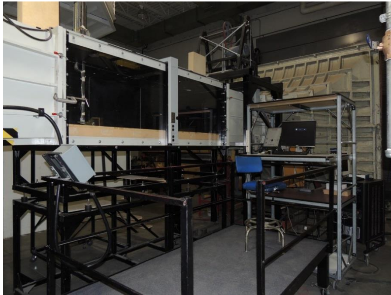
Figure 10. Bill James Wind Tunnel (8 ft. test section and upstream contraction shown)
