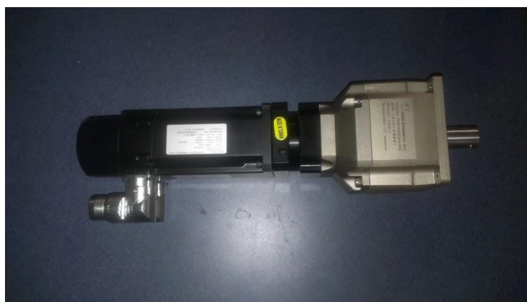
Figure 15. Kollmorgen AKM23C Servomotor with 100:1 gearbox
