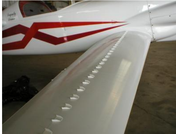
Figure 2. Vortex generators on a Dragonfly wing
